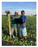
Graduate students download soil data collected using Time-Domain Reflectometry (TDR) sensors.
